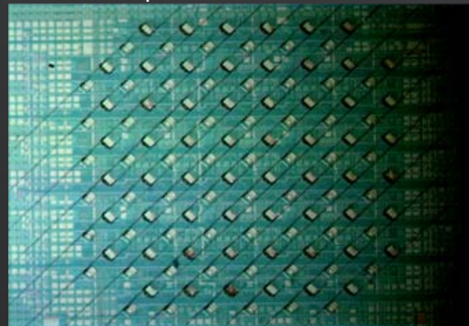
CMOS chip with memristive devices
