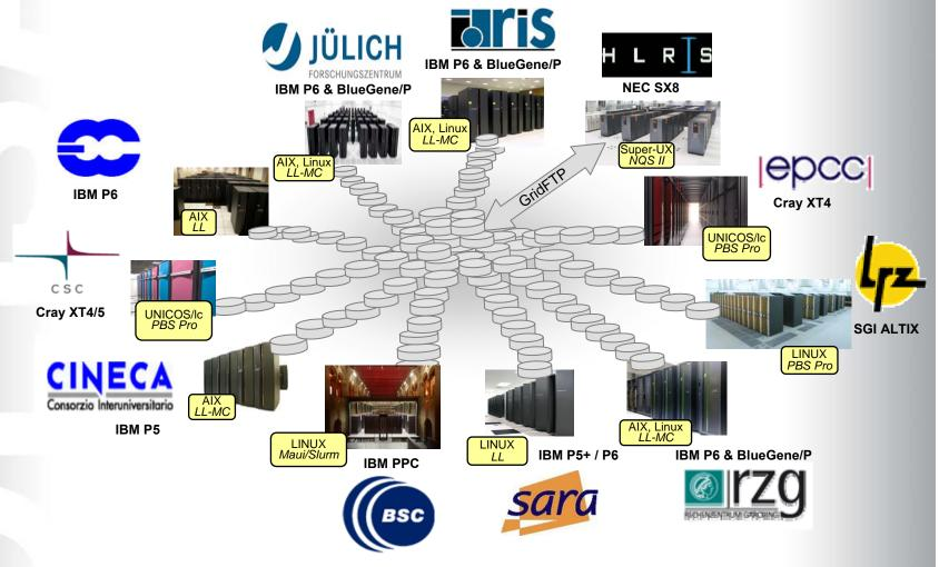
Global transparent file system based on the Multi-Cluster General Parallel File System (MC-GPFS of IBM)
