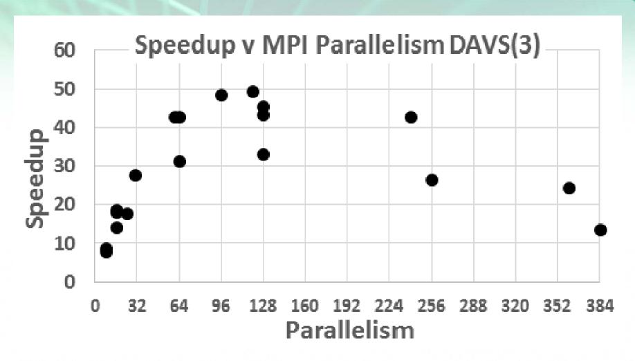
Speedups for several runs on Tempest from 8-way through 384 way MPI parallelism with one thread per process. We look at different choices for MPI processes which are either inside nodes or on separate nodes
