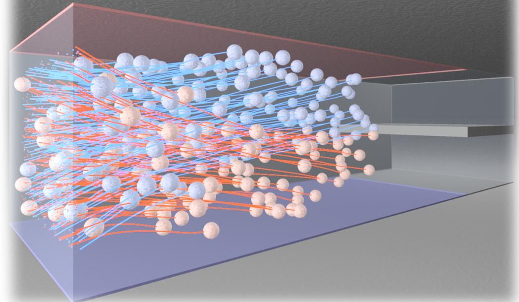
Positive and negatively charged particles in flow subjected to transversal electric field
